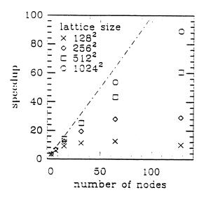
Figure 1: Speedups on the Symult 2010 for self-labeling.
